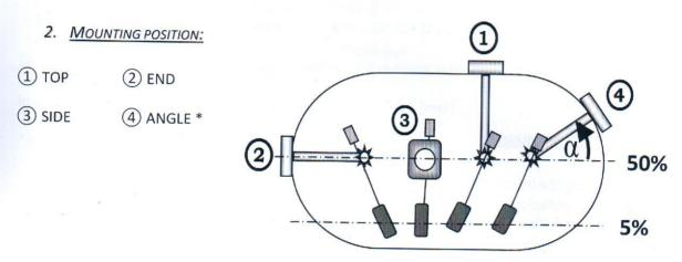
(\*) angle to be specified from horizontal pane (positive above horizontal, negative below)
